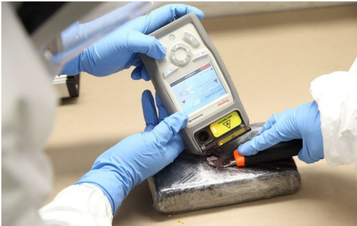
Customs officers using the FirstDefender at an inspection facility to identify an illicit substance
